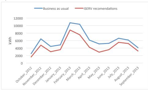
represented in the figure on the right and include AHU control improvement, turn off equipment when not in use and adjust the cooling and heating demand for the real requirements of the building. The estimated result of this measures could represent a reduction of 27% in the HVAC systems and consequently in the electricity use, without major investments. The reduction of the total annual building energy use can be reduced to 14 kWh/m².year.
