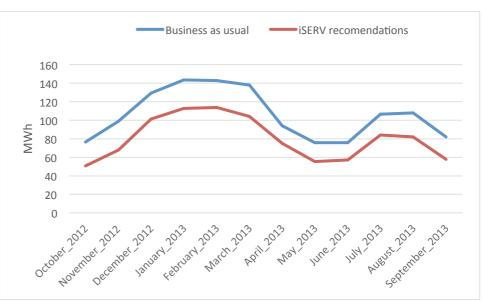
equipment. This measures are represented in the figure on the right and include AHU control improvement, turn off equipment when not in use and adjust the cooling and heating demand for the real requirements of the building. The estimated result of this measures could represent a reduction of 25% in the HVAC systems and consequently in the electricity use, without major investments. The reduction of the total annual building energy use can be reduced to 19 kWh/m².year.
