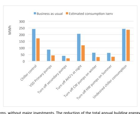
reduction of 41% in the HAVC systems, without major investments. The reduction of the total annual building energy use can be reduced to  $563.7 \text{kWh/m}^2$ . year, representing electricity savings of 29% from the electricity use.
